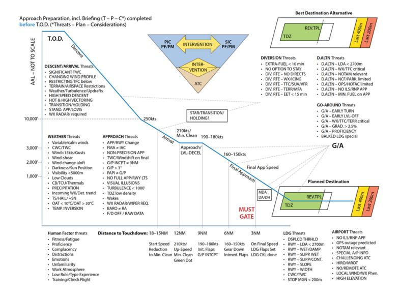
Approach briefings should be finished before top of descent, whenever feasible. On very short flights, it might be useful to already complete parts of the approach briefing on the ground. Approaches should be delayed if not being fully prepared. Approach preparations should include the following:
