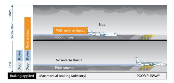
Pilots should be aware they may not be used to full braking or full reverse. They should plan accordingly and be prepared to ignore environmental restrictions (e.g. noise) when required for safety. GAPPRE 4.2
